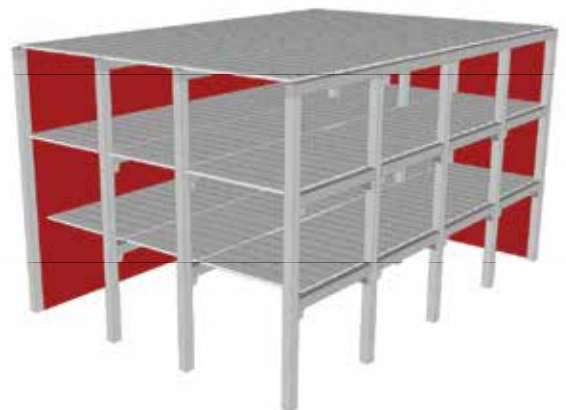
Figure 2.5 Shear wall configurations to be avoided due to the fact that they are not symmetrical in plan with respect to two orthogonal axes.
