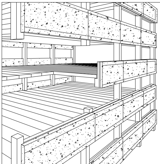
Figure 4.7 Load-bearing spandrel beams
